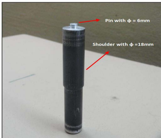
Fig. 4: FSW Tool (X38 tool steel)
